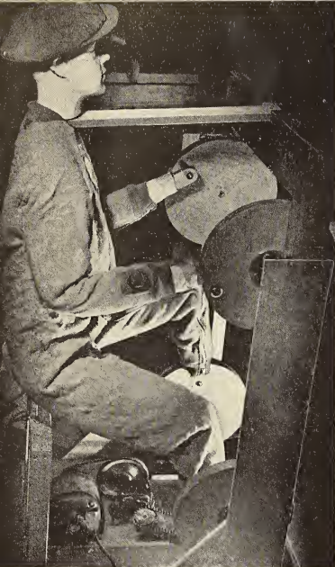
Meet "Horatio"—the mechanical man who works 24 hours a day testing flying suits.
